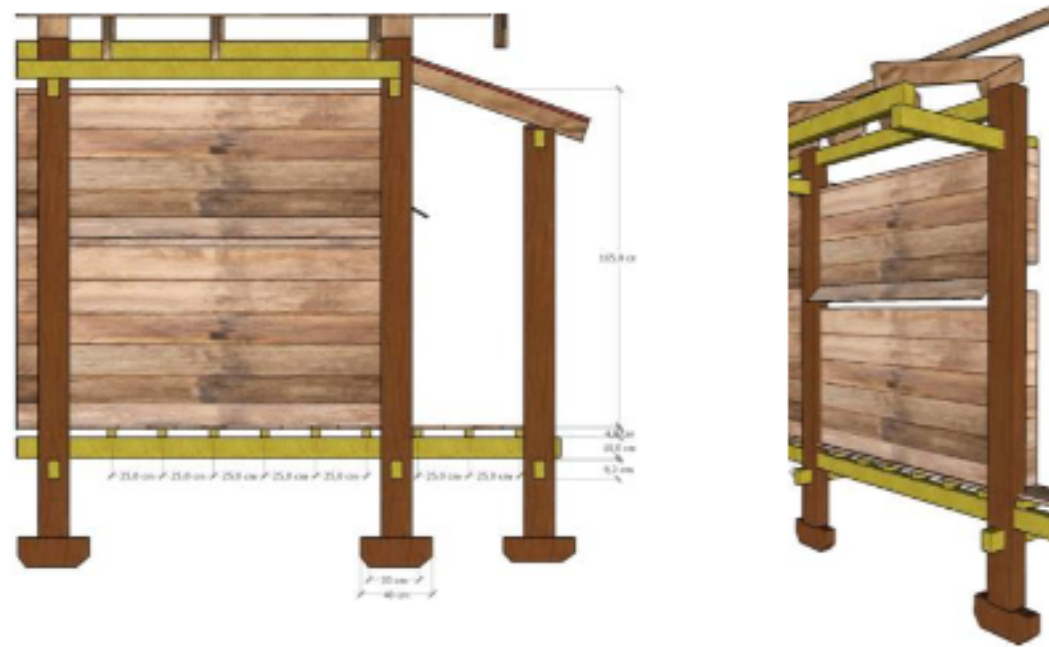
Figure 8. Construction Details of Type 1 Board Walls on the Front and Side Source: Personal Sketch, 2021
