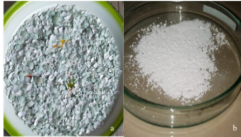
Fig. 2 Egg shells, the basic material for producing catalysts: a. egg shell; b. \text{CaO}/\text{Na}/\gamma\text{-Al}_2\text{O}_3
