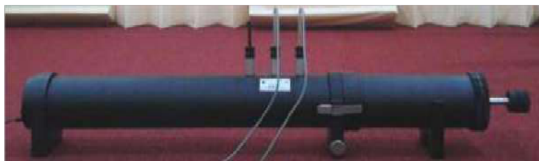
Figure 2 Impedance tube type 4206
