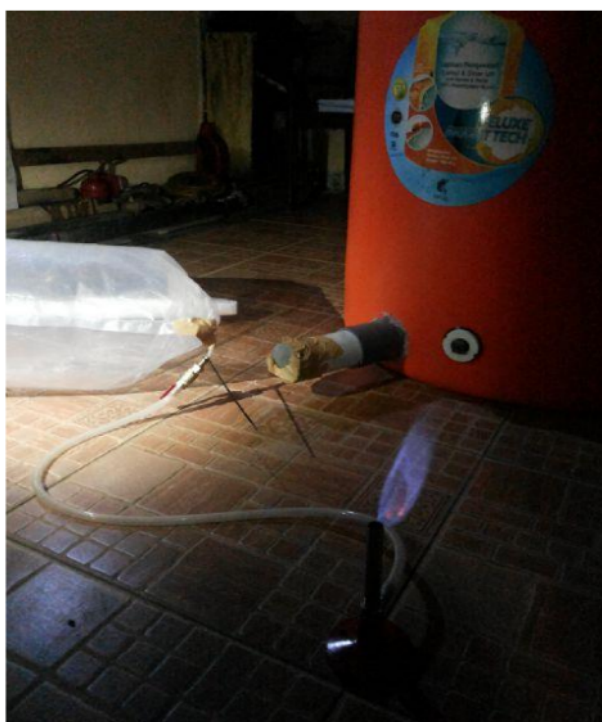
FIGURE 4. Biogas combustion test
