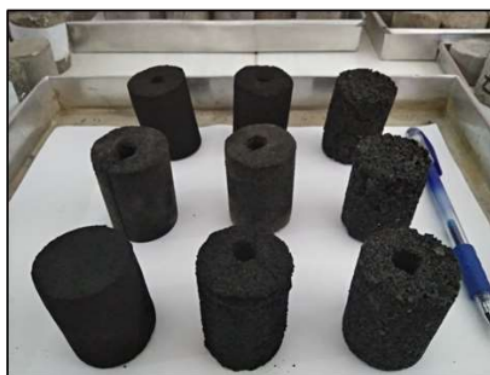
Figure 2. Briquettes of 28, 65 and 80 mesh in different composition.
