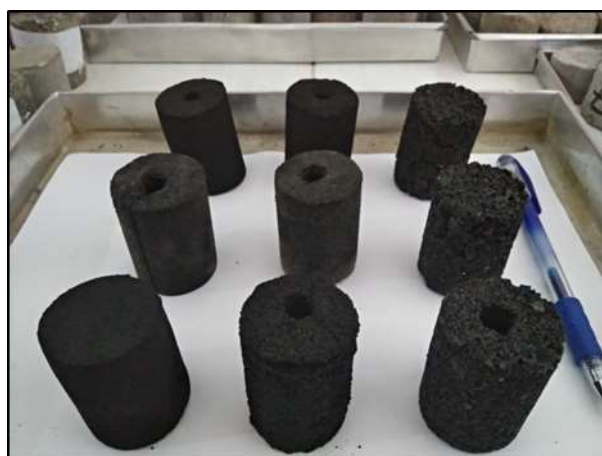
Figure 2. Briquettes of 28, 65 and 80 mesh in different composition.
