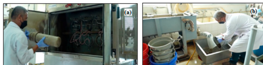
Figure 5. (a). The pulp from the first stage was put into the CRS AB rotary digester reactor with a capacity of 6 L and cooked at a temperature of 165 °C for 60 min. To reach the maximum temperature the pulp is held for 90 min, hence, the total time in the cooking process is 150 min; (b). The cooked pulp is then separated from the black liquor, washed and then screened to separate it from the residue.
