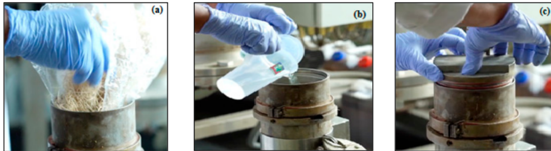
Figure 4. (a). EFB fiber (first sample and second sample) with a length of 2–3 cm and a mass of 300 g was inserted into the rotary digester tube (b). Addition of 1 N sulfuric acid, 0.4% sulfate pre-hydrolysis with a ratio of 1:5 ( w/v ); (c). EFB fiber was cooked at 130 °C for 60 min (time to reach maximum temperature was 60 min and held for 90 min).
