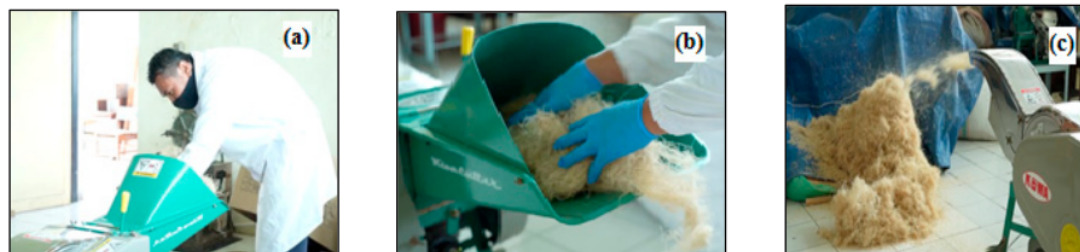
Figure 3. (a). WEFB fiber and SEFB fiber are cut using a cutting machine; (b). The cutting process is performed manually slowly to obtain good cutting results; (c). The long fibers that have been cut have a size of about 2–3 cm.
