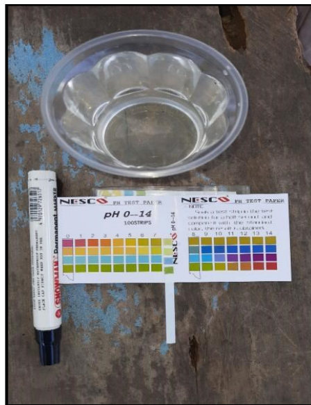
Figure 2. Measurement of pH and Observation of Physical Properties of Shallow Wells
