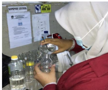
Gambar C.4 Penambahan Air kedalam botol VCO dan emulsifier
