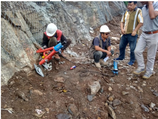
Gambar.16 Uji Tarik Angkur Pin
