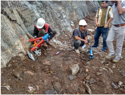
Gambar.16 Uji Tarik Angkur Pin
