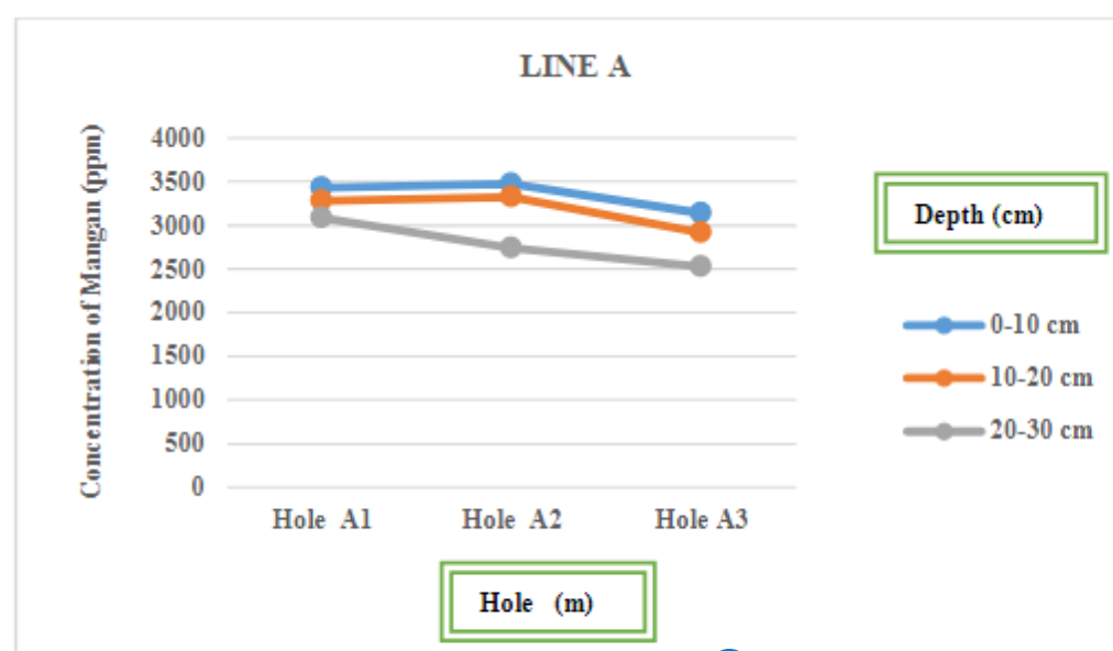
Figure 2. Graph of lateral analysis result of Manganese (Mn) heavy metals for line A and sampling points (A1, A2 and A3) at the depth of 0-10 cm, 10-20 cm and 20-30 cm, in the soil around Antang landfill of Makassar.
